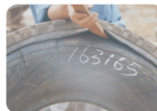
Puncture and Delamination
