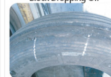
Shoulder Damage & Pattern Block Dropping Off
