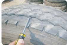
Tire Crown Abrasion Under Low Air Pressure
