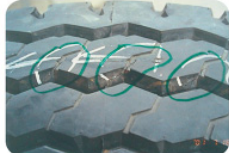
Tire Crown Pattern Breaking Damage
