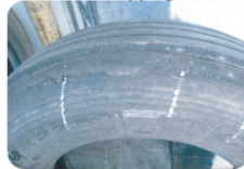
Shoulder Damage & Pattern Block Dropping Off
