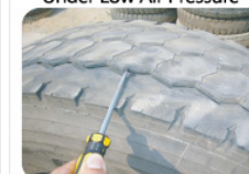
Tire Crown Abrasion Under Low Air Pressure
