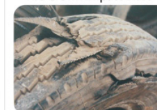
Tire Crown Impact Blast
