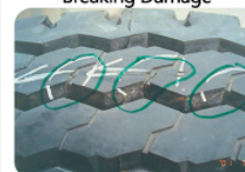
Tire Crown Pattern Breaking Damage
