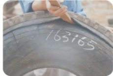
Puncture and Delamination
