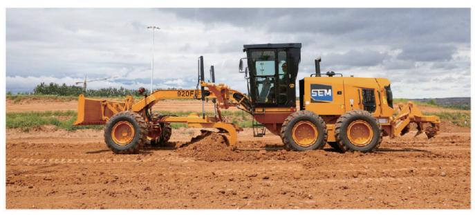
Typical applications such as ground leveling and trenching, slope scraping, bulldozing, snow removal, loosening, distribution, mixing and land reclamation, etc. It is an important equipment in the construction of mine construction, road construction, water conservancy construction and farmland turning and leveling.
